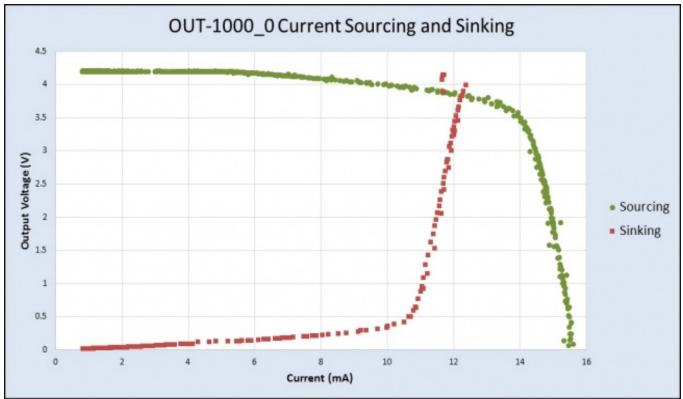
For example, if the connected circuit is expected to pull 14mA of current, the OUT1000 will only be able to provide a maximum of 3.5V, even if you try to set it to a higher value.
