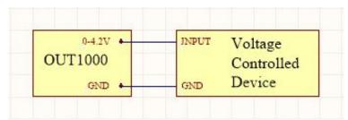
Some devices may require an analog voltage as a control input. The OUT1000 supplies a fixed voltage up to 4.2V, which can be used to control such devices.
