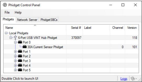
The Phidget Control Panel will list all connected Phidgets and associated objects, as well as the following information:
