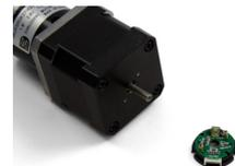
Get the encoder disk and hex key. Do not touch the surface of the encoder disk, as your fingerprints could affect the operation of the optical sensor. Place the encoder disk on the rear shaft of the motor with the metal coupler facing outward. Slide the encoder disk until the surface of the disk is approximately 1.5mm from the optical sensor on the PCB. Use the hex key to tighten the set-screw on the coupler of the encoder disk.
