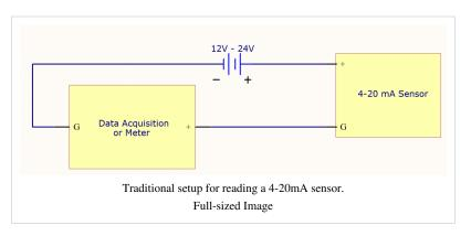
movement, and would output 20mA when the sensor is moving at the maximum velocity it can sense. 4-20mA sensors are usually expensive and intended for industrial purposes. There are often less expensive 0-5V analog versions available.
