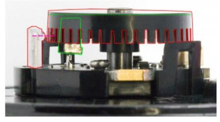
Take the plastic cap and align the hole with the white connector. Press the cap on so that the tabs on either side click in.
