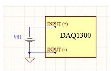
The DAQ1300 can be used without additional circuitry to detect the presence of a voltage on a line (from a power source or a signal), by wiring the input terminals to the line and its corresponding ground.
