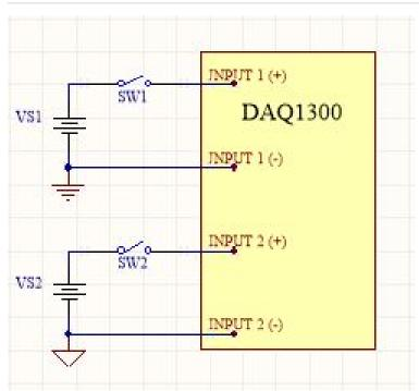
All inputs on the DAQ1300 are isolated from one another, so a variety of signals from different sources can be monitored with a single device.
