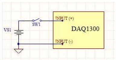
To interface a switch with the DAQ1300, an external voltage source must be provided to pull the input HIGH.
