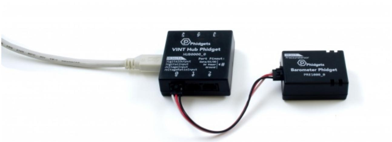
1. Connect the PRE1000 to the VINT Hub using the Phidget cable.
