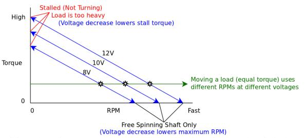
Building on the previous example, lets say that we're using a motor controller that enables switching between three voltage levels: 8V, 10V and 12V. Please note that while it's acceptable to provide less than the rated voltage, you should not supply a motor with significantly more than the rated voltage. In this example, assume the motor is rated for 12V.
