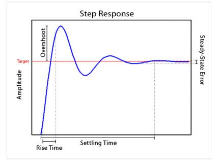
• **Settling time** is how long it takes for the oscillations in the system to
