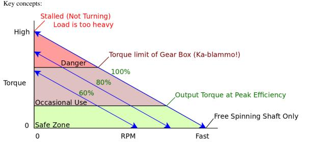
The above graph is separated into three sections based on the size of the load that the motor is working against (and consequently the amount of torque being applied).
