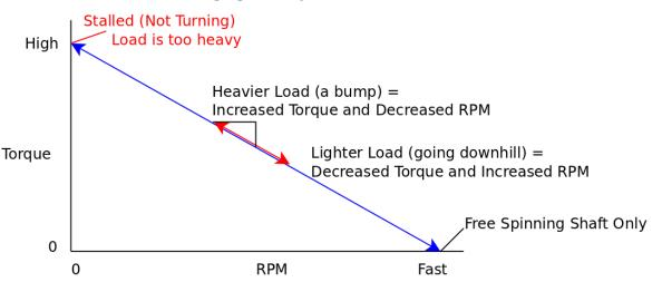
In this case, the PWM duty cycle is held constant, but the load is changed (in this example, because of difficult terrain). When this happens, both RPM and torque change, and we're unable to change torque or RPM individually to compensate and keep moving at a constant speed. If we combine the concepts of these previous two graphs, we can devise a method to control the RPM for a changing load.
