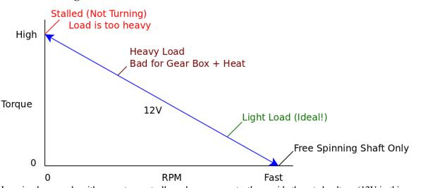
In a simple example with no motor controller, when you constantly provide the rated voltage (12V in this example), the motor will try to spin as fast as it can based on the magnitude of the load resisting it. The blue line in the above graph illustrates the range of torque/speed values that the motor could operate at depending on the magnitude of the load.
