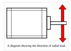
mounted close to a tire, if the tire is wide it will still have considerable leverage on the motor's shaft. In applications with high potential for radial load, it would be advisable to drive the axle indirectly.
