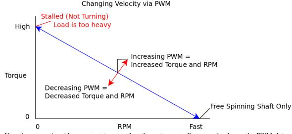
Now, in a scenario with a constant torque value, the motor controller can only change the PWM duty cycle. By increasing the duty cycle, you increase both the torque and the RPM (as shown by the black line vector components). In this case we cannot change RPM and torque individually.
