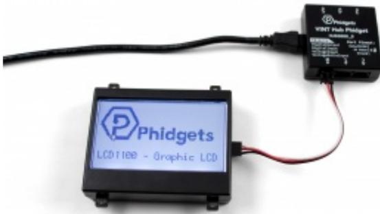
1. Connect the LCD1100 to the VINT Hub using the Phidget cable.
