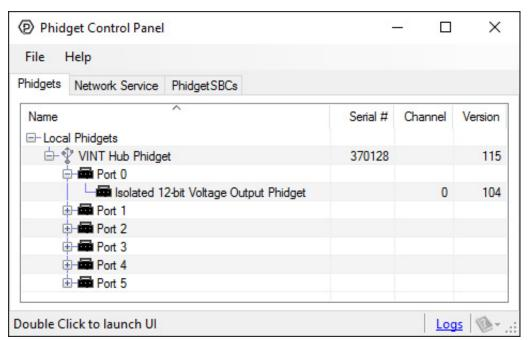
The Phidget Control Panel will list all connected Phidgets and associated objects, as well as the following information:
