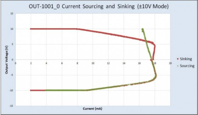
For example, if the connected circuit is pulling 13mA of current, the OUT1001 will only be able to provide a maximum of 4V (in 0-5V mode), even if you try to set it to a higher value.
