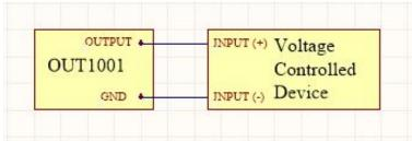
Some devices may require an analog voltage as a control input. The OUT1001 supplies a fixed voltage up to  $\pm 10$ V, which can be used to control such devices.
