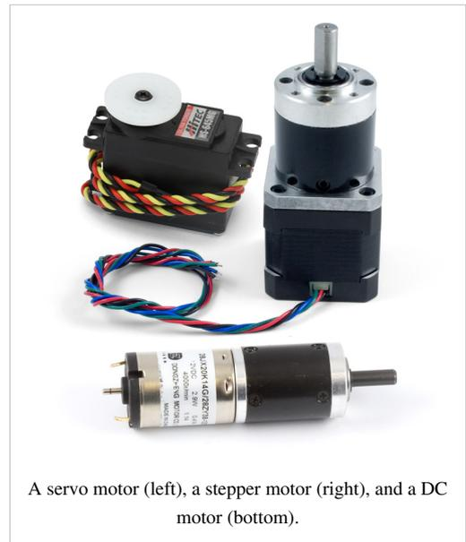
A servo motor (left), a stepper motor (right), and a DC motor (bottom).
