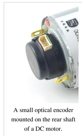
A small optical encoder mounted on the rear shaft of a DC motor.
