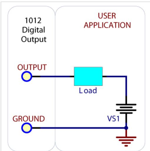
Switching a circuit with an open collector digital output.
