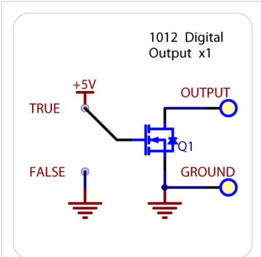
A simplified schematic showing of a Phidgets open collector digital output.
