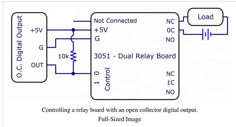
control line to become grounded. Since this is the opposite of the usual operation of a relay board, you'll have to hook your load up to the **normally closed** terminal if you want the load to be powered when the digital output is turned on, or connect it to the **normally open** terminal if you want the load to turn off when the digital output is turned on.
