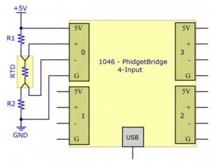
This diagram illustrates how to connect the RTD to the PhidgetBridge with
