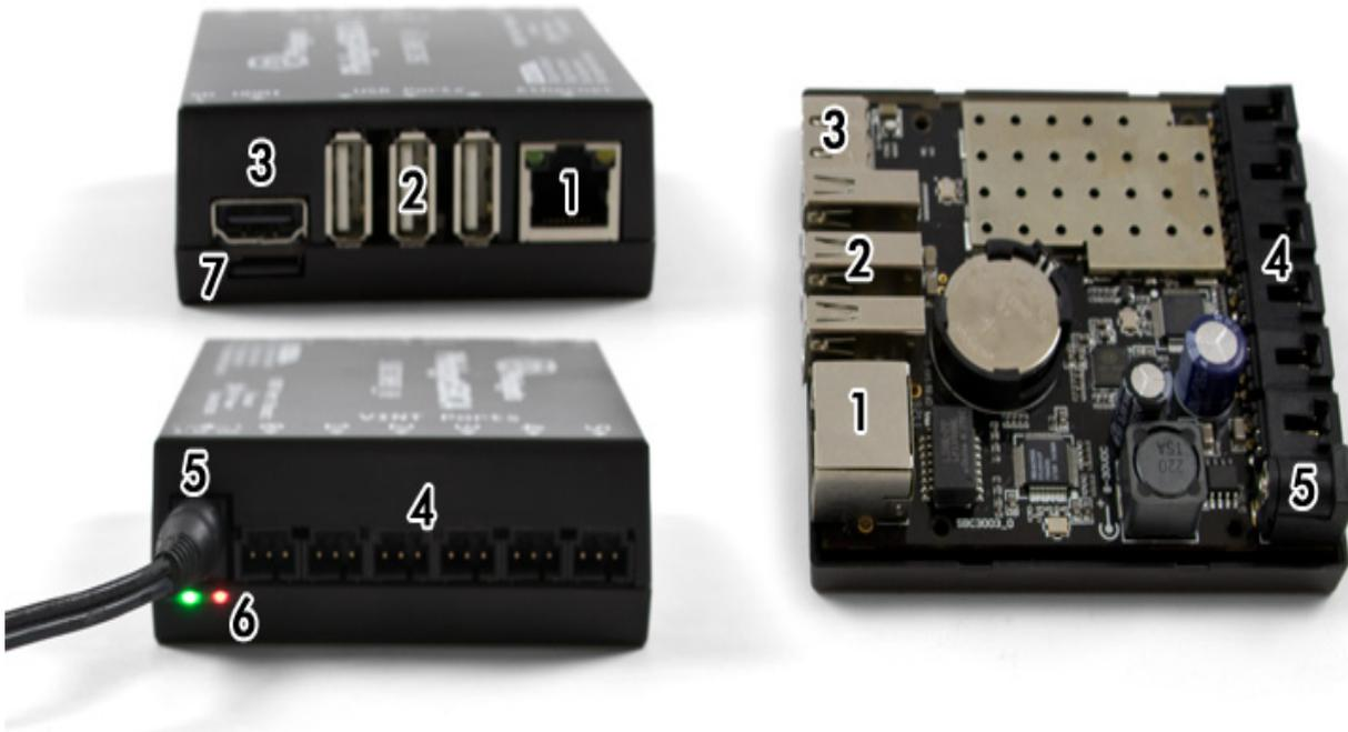
1. The Ethernet port is used for network connectivity to the SBC. This enables network access to the SBC as well as any connected Phidgets through the Phidget Network Server. Alternatively, a Wi-Fi USB adapter can be used for wireless network connectivity.
