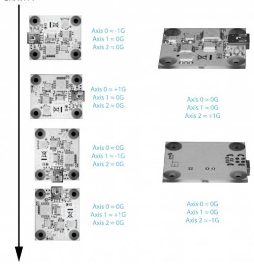
When working with an accelerometer it is important to know which is the positive and negative direction on each of the axes. This can be determined by orienting the accelerometer along each axis and checking the output. The above image shows what the axis readings should be for each orientation of the 1043.
