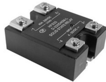
A "hockey puck" SSR, so named because of its thick shape and black color. They are specifically designed to switch either AC loads or DC loads, but never both.
