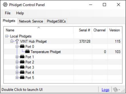
The Phidget Control Panel will list all connected Phidgets and associated objects, as well as the following information:
